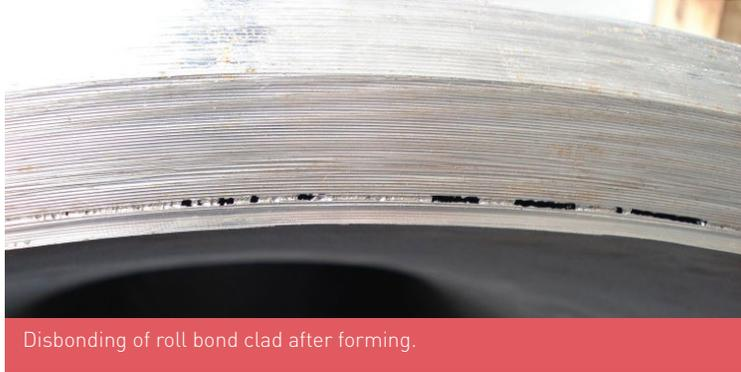
Disbonding of roll bond clad after forming.
