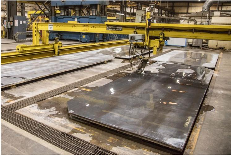
*Automated ultrasonic testing (UT) scanning of up to 100% of clad plate surface area in Mt. Braddock, PA facility.*
