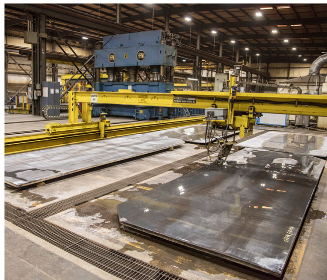
Ultrasonic testing of clad plate
