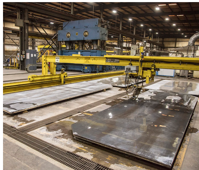
Ultrasonic testing of clad plate
