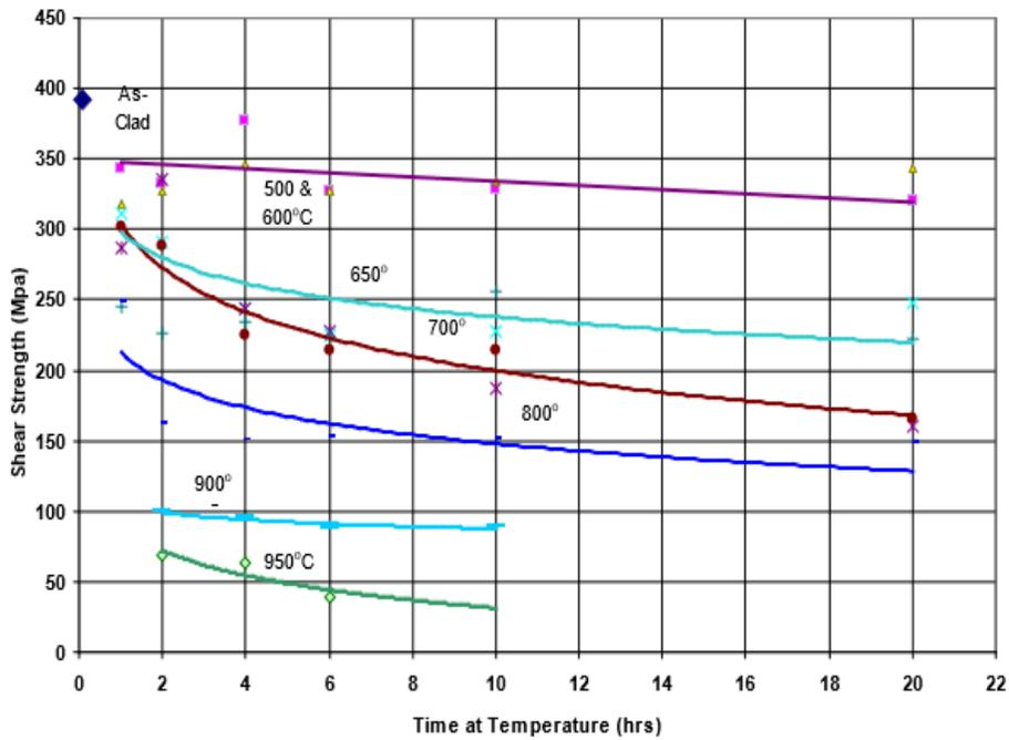
**FIGURE 6: SHEAR STRENGTH OF TITANIUM-STEEL CLAD VS. TIME AT TEMPERATURE [17]**
