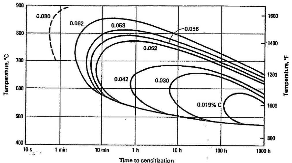
**FIGURE 1: TIME-TEMPERATURE-SENSITIZATION (TTS) OF 304 STAINLESS STEEL, EFFECT OF CARBON<sup>[14]</sup>**
